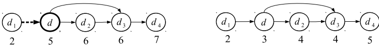
Fig. 2. Relocation of distances after the insertion of the new transition entering d
