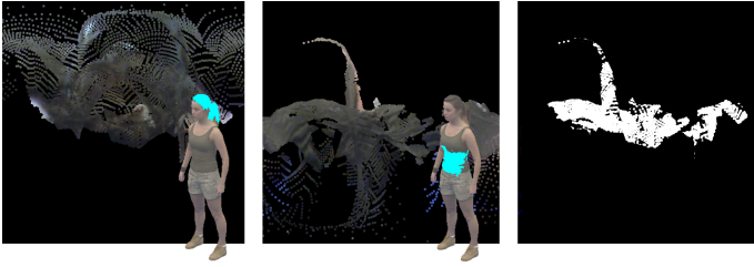
Fig. 2. Local irradiance estimates (left and centre) for two materials (polar projection). On the right, the intersection between the two irradiance estimates, Q_{ij} . Also shown are the positions of the materials on the mesh surface, highlighted in cyan.
