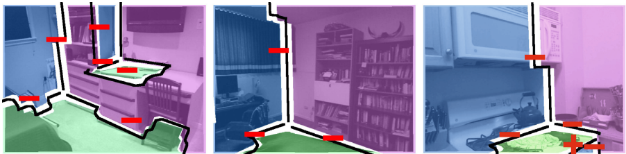
Fig. 7. Surface connection graphs of scenes automatically obtained from a single image. Our method infers a parse of the scene in terms of large vanishing-point-aligned regions and the edges between them (convex: +, concave: -).
