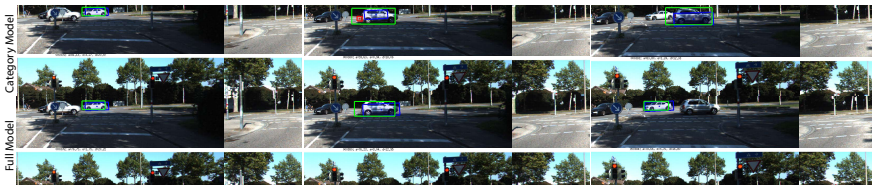
Fig. 5. The tracking results on KITTI03. “Category Model” fails to track the target and switches to the occluder, while our full model is able to recover from occlusion and track the correct target.
