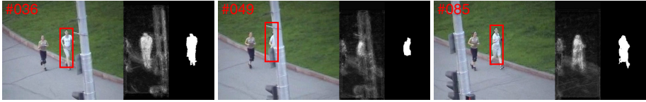
Fig. 2. Occlusion handling on the Jogging sequence. The index is specified in the top-left of each frame, and the two figures between each frame are the corresponding outputs of the pixel-level RFs and labels x_i , respectively. The occlusion is detected from the Frame #049, from which point the RFs stop updating until the target moves out of occlusion.
