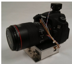
Fig. 7. Our prototype Motion Invariance camera, based on an unmodified Canon 60D with a modified 100mm Macro IS lens. The hot shoe triggers our Texas Instruments MSP430F2618 microprocessor (located inside the metal box) to start parabolic lens motion.
