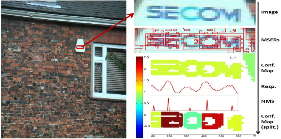
Fig. 4. Error-connected component slitting by sliding window model with the CNN classifier
