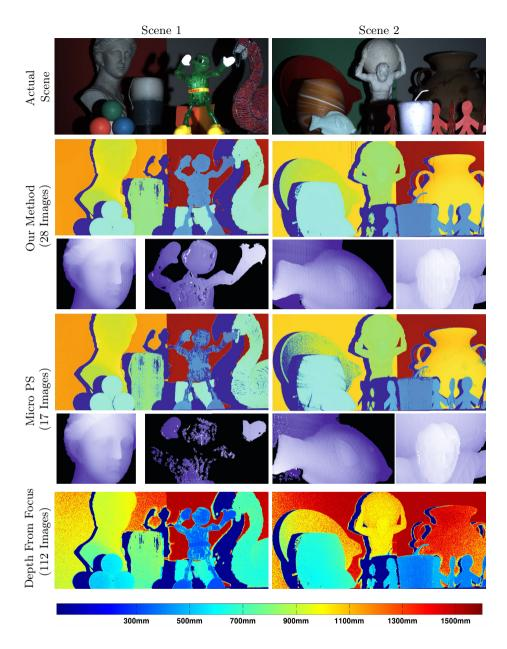
**Fig. 7.** Recovering Depth: Our structured light algorithm is able to recover depth maps for scenes containing challenging objects over an extended working volume with relatively few images. The insets for our method and micro phase shifting show (rescaled) depth maps for small parts of the scene. Many fine details on objects like the scales on the soap fish are successfully resolved.
