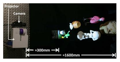
Fig. 6. Experimental Setup: With a small, 500 lumen DLP projector and a small number of images, we are able to scan scenes over a large working volume to recover accurate depth maps and perform illumination separation.
