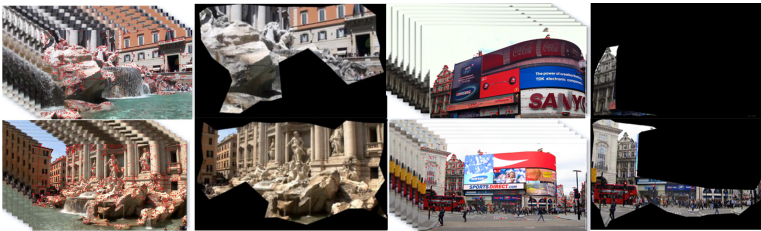
Fig. 4. Static content prior from video fragments. First and third columns depict SIFT features matches among neighboring frames as red dots. Second and fourth columns depict the concave hull defined by detected features not overlapping with the existing dynamic content prior.
