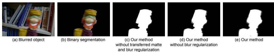
Fig. 4. Effect of each matting component on the alpha matte result. (a) Original image. (b) Binary segmentation. (c) Alpha matting without the transferred matte and motion blur regularization. (d) Alpha matting without motion blur regularization. (e) Proposed method.
