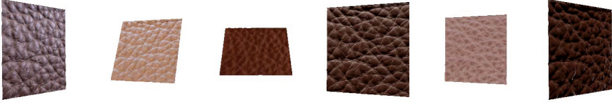
Fig. 3. Examples for synthesized images of the same material sample demonstrating the large variation under different viewing and illumination conditions
