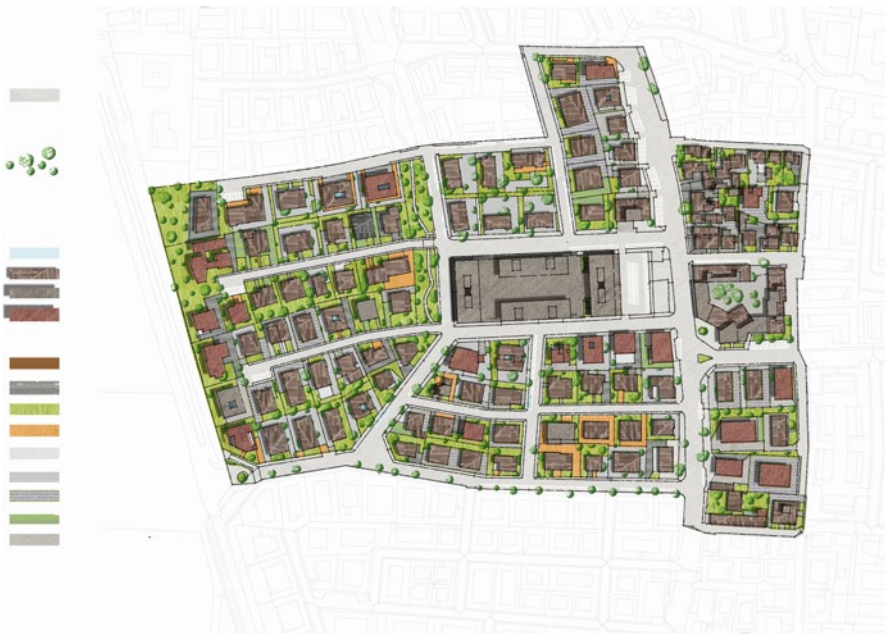
Fig. 8.11 Intervention 2 +summary of intervention 2 Modify the albedo of sidewalks and parking lots. Modify the reflectance of sidewalks and parking lots
