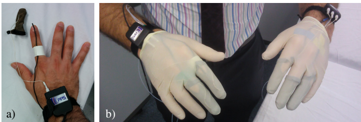
Fig. 1. a) DRE: a Micro 6DOF position sensor coil on the nail of the index finger with a capacitive pressure sensor next to it. b) BVE on GTAs: a consultant wearing position sensors (index and middle fingers of both hands) with five pressure sensor sheaths (one additional next to middle finger of external hand).
