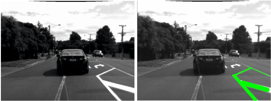
Fig. 8. Detection results for lane markers in real-world images. Left: Original images. Right: Detected lane markers.
