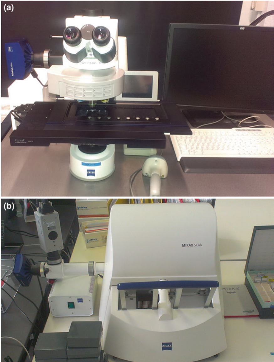
Fig. 2.1 a A Zeiss AxioVision setup with a mounted camera and robotic stage (courtesy of HistoGeneX). b A 3DHitech high-volume slide scanner (courtesy of HistoGeneX)
