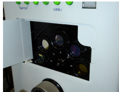
Fig. 7. Filter turret and band-pass filters in the xenon lamp system
