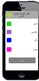
Fig. 3. Color Matching Interface. It shows the detected color and 4 matching colors that go with it
