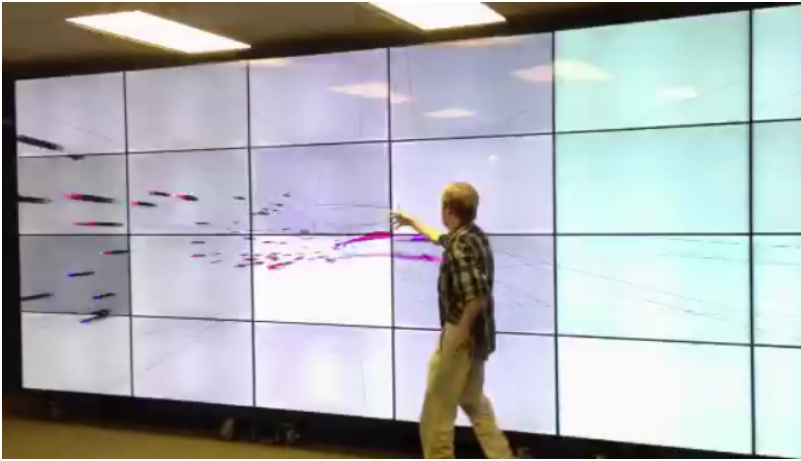
Fig. 4. Users can improvise real-time sonification and visualization based on their location, movement, and gesture. They can change multiple mappings via the scripting language.
