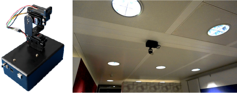
Fig. 4. Visual Feedback Robot (left) and mounted on living room ceiling (right)
