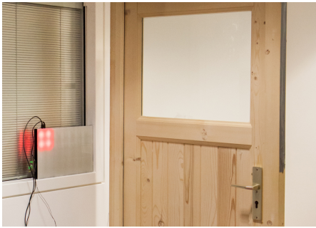
Fig. 8. The minimalistic feedback shows the state of the door - which is currently locked (red)
