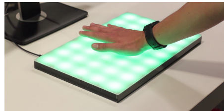
Fig. 7. When a gesture is recognized successfully, the device lights up in green. Moreover, it is possible to indicate unrecognized or unsupported gestures by lighting up in red.
