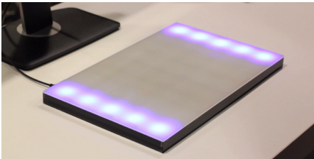
Fig. 6. Interactive regions are visualized with a glow effect. When the hand moves over the corresponding region, an application-specific action is triggered (e.g. scrolling in the image viewer).
