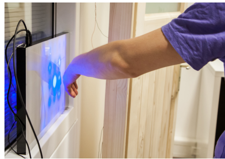
Fig. 9. The extended feedback also indicates when a hand approaches the gesture-recognizing surface
