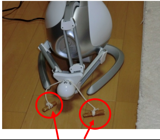
Dog treats were attached to the haptic device at the dog site.
