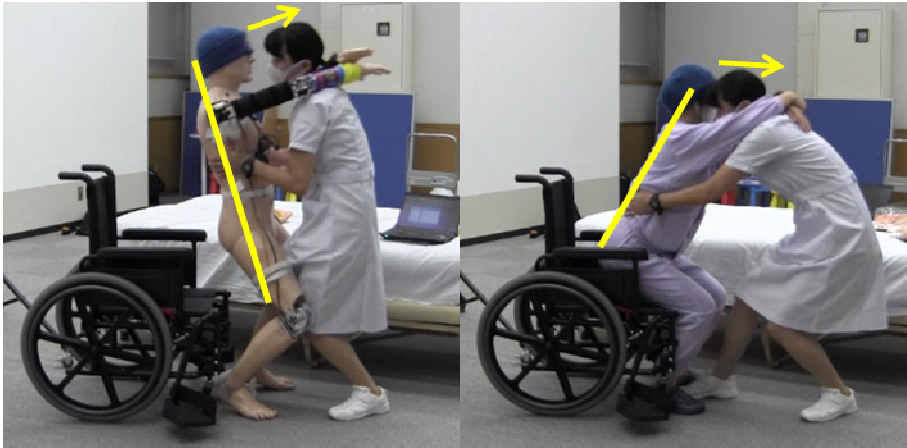
Fig. 3. Comparison of robot and human, bending angle of back
