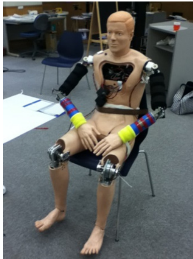
Fig. 1. Robot patient for wheelchair transfer practice
