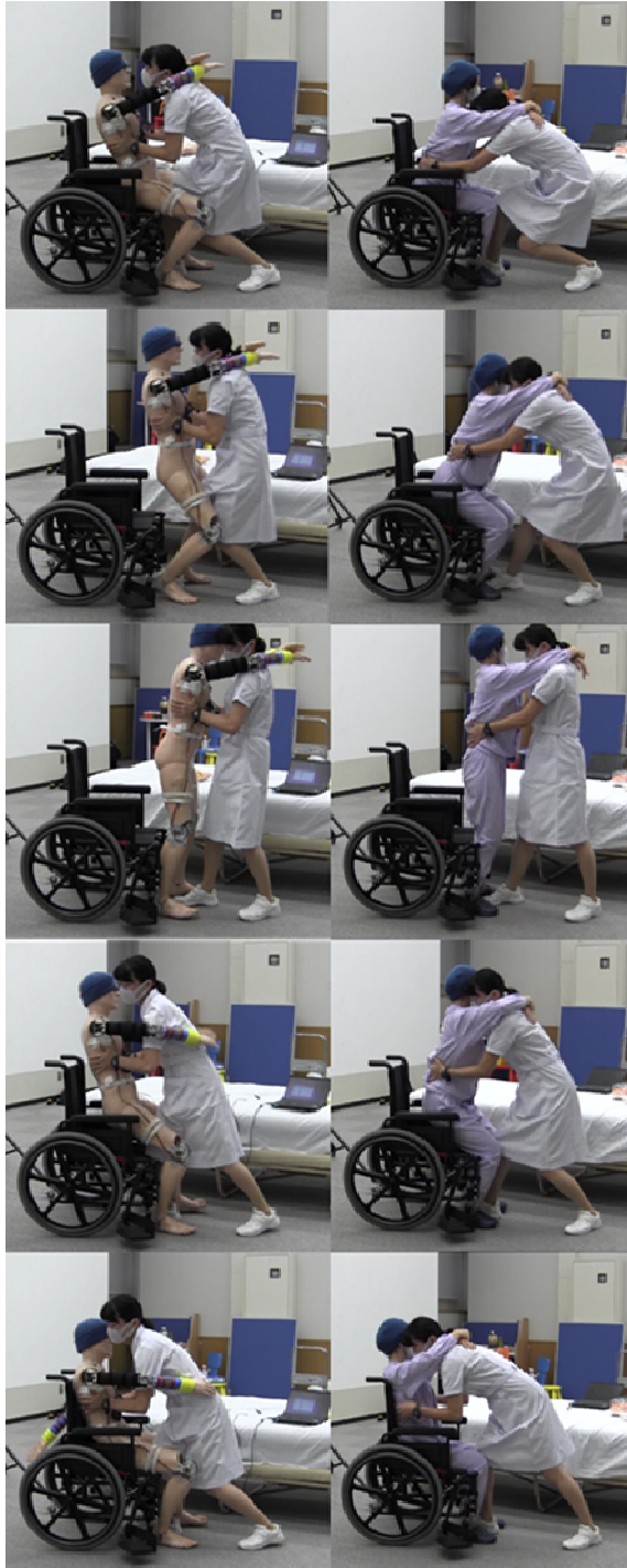
Fig. 4. A sequence of actions of wheelchair transfer methods (Left robot and human right)
