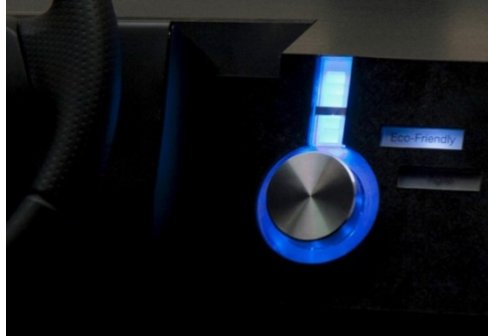
Fig. 4. UX Component: Prototype of a natural energy interface in an electric vehicle
