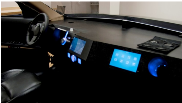
Fig. 5. UX Product: Natural energy interface integrated into the dashboard of an electric vehicle
