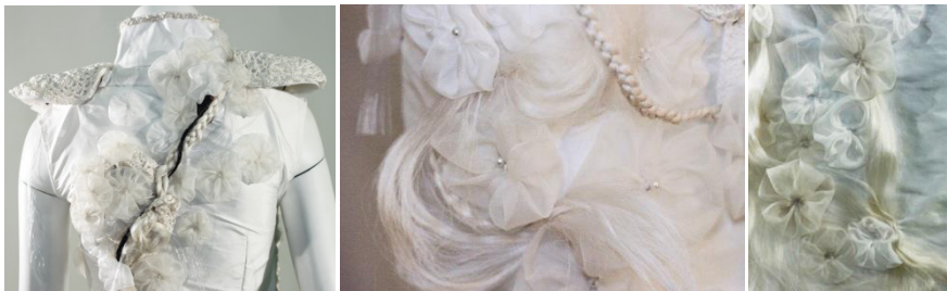
Fig. 6. The shoulder shells house the 2 servomotors that pull on the organza flowers
