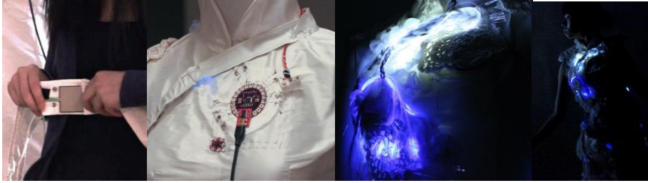
Fig. 5. (Left) The breath chest band containing the squared FSR sensor transmits pressure data to the Lilypad Arduino microcontroller. (Right) The LEDs illuminate based on the values sent from the Lilypad Arduino microcontroller board.
