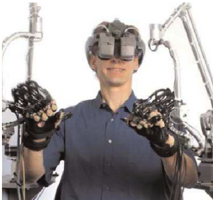
Fig. 1. CyberGrasp ™ haptic glove designed by Immersion Corporation
