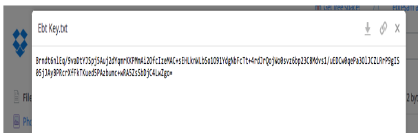
Fig. 9. AES key is encrypted by public key and stored in Dropbox
