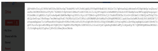
Fig. 8. User text file is encrypted by AES key and stored in Google Drive
