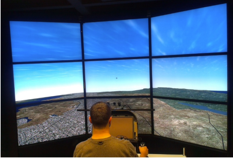
Fig. 3. Fixed-base flight simulator, consisting of nine panels and a field-of-view of 105^\circ \times 100^\circ . Here the Outside View is shown. During the experiment, visual disturbances were experienced in the roll-axis around the horizon, that our participants were instructed to compensate for with the provided joystick.
