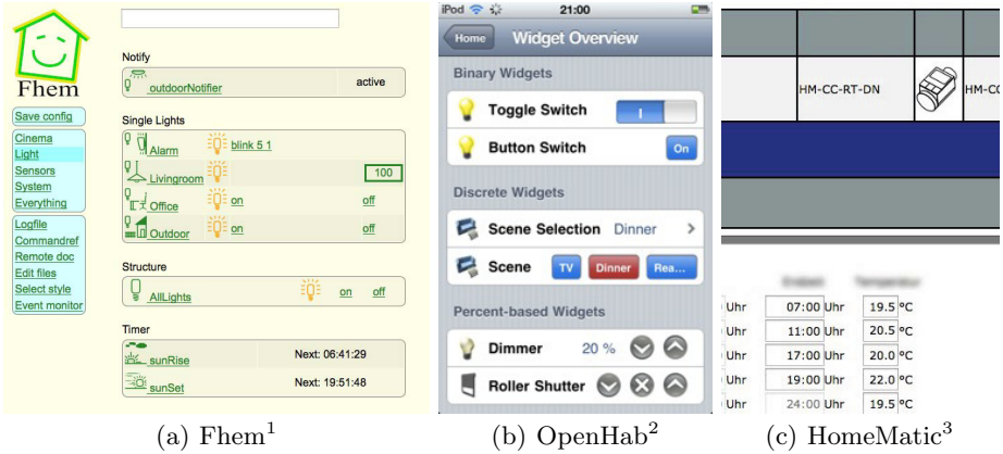
Fig. 1. Example of user interface based on list views
