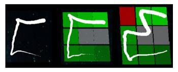
Fig. 5. Bottom right corner feedback: on the left side the gesture before its completion (A button release), in the middle the correct gesture and on the right side a gesture with an error
