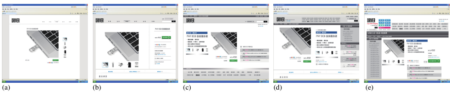
Fig. 1. The experimental web pages of Experiment 1. The calculated visual complexity score by the Quadtree decomposition method [25] is: (a) 2.23, (b) 3.70, (c) 5.99, (d) 7.90, (e) 9.88, respectively.
