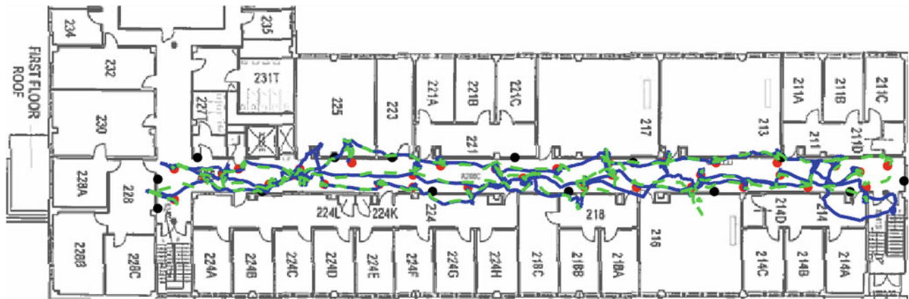
Fig. 2 Trajectory in the hallway estimated without calibration (solid blue line) and with the considered calibration model (green dashed line)
