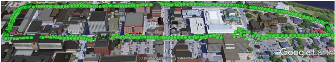
Fig. 9 SPP and INS loosely-coupled integration results
