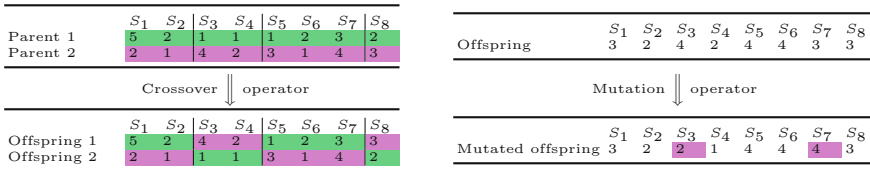
Fig. 1. Solution representation using vectors of integers. Example of the crossover (left) and mutation (right) operators.
