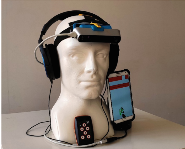
Fig. 1. Components of the ETA system, consisting of a depth camera, an Android OS smartphone, a pair of headphones and a remote controller.
