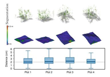
For every artificial plot, our model efficiently filters out the vegetation points. Moreover, the reconstructed surfaces are placed at a mean distance of 2 cm from the terrain model produced with Meshlab, except in large occlusions where ground points are missing and where the reconstructed surface is approximated from the surroundings.
