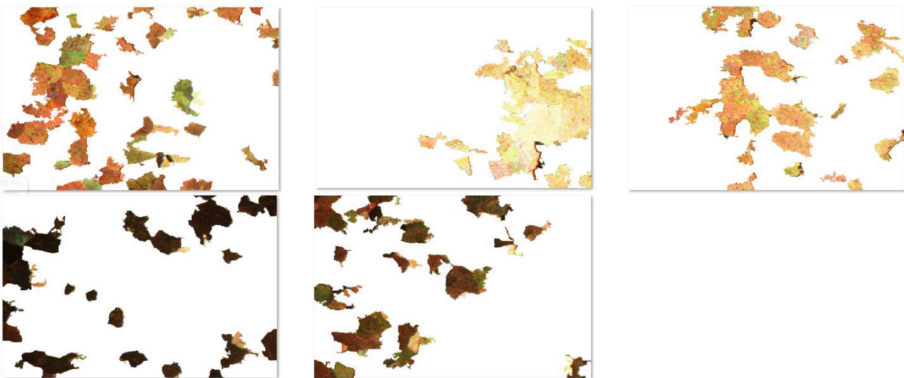
Fig. 7. Groups of the most characteristic rock fragments with a coherent grain color (dolomite from the Beskid Mountains) - estimation consistent with visual assessment.
