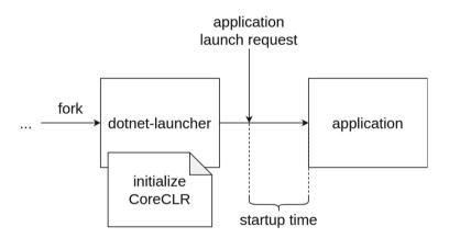
Fig. 2. CoreCLR initialization in candidate process
