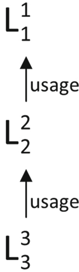
Fig. 1. One-to-one relationship between lots. This is the simplest relationship that we can find in the manufacturing industry. In principle, a solution for dealing with this type of relationship is quite simple and can be implemented efficiently in a wide range of database systems, including those databases making use of the traditional model.
