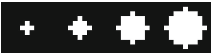
Fig. 10.3 Some circle masks. These are examples of the circular masks used by the segment sensor algorithm to determine line width. The circles displayed here correspond to diameters of 2, 4, 6 and 8 pixels. The masks are squares with an odd number of pixels as they are centered at a unique pixel
