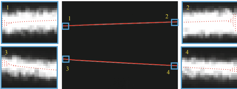
Fig. 10. Multiple light stripe center extraction based on Hessian matrix
