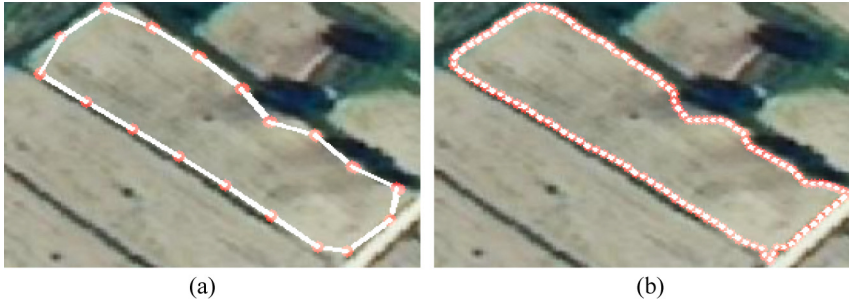
Fig. 8. Information extraction results at different sampling intervals. (a) Line segments separated by 30 pixels; (b) Line segments separated by 5 pixels.
