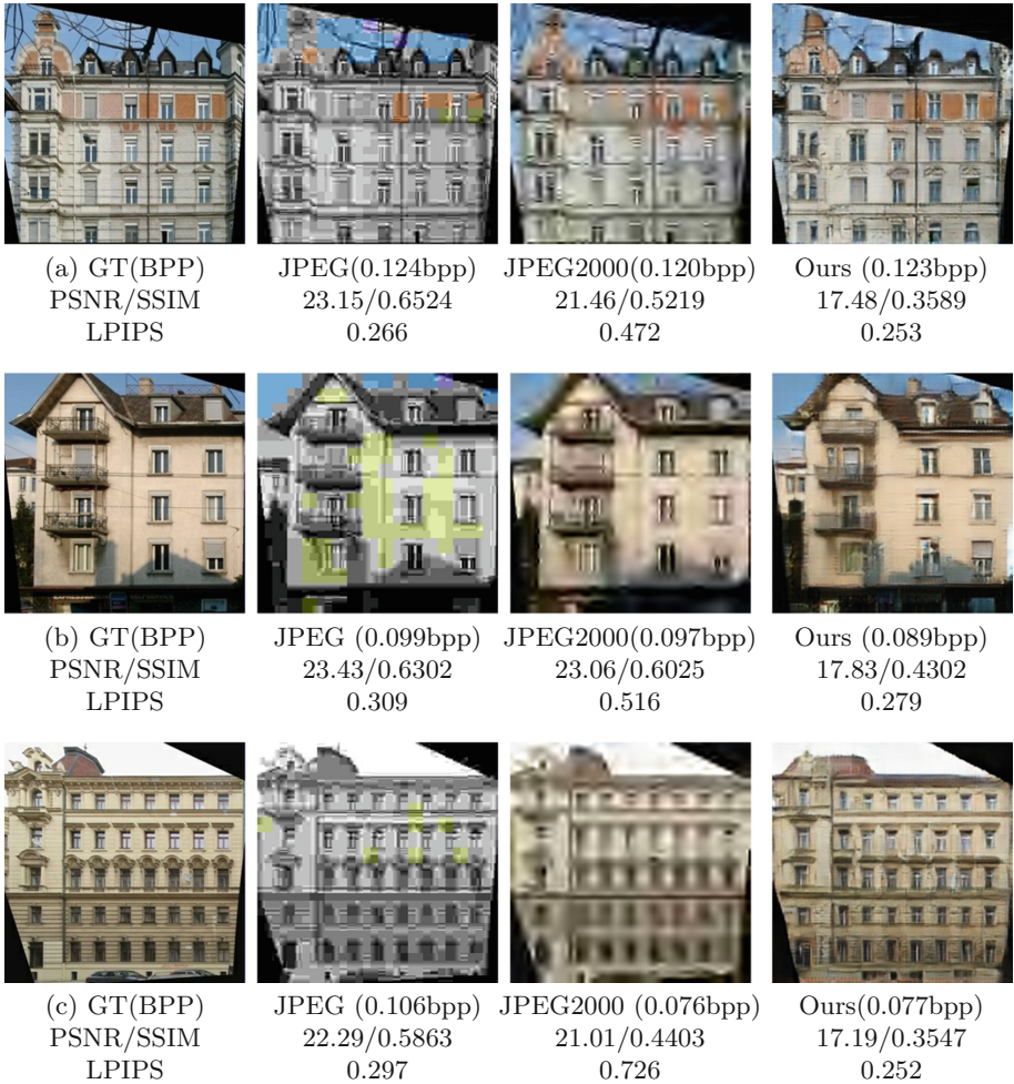
Fig. 4. Subjective comparison on several images compressed by JPEG, JPEG2000 and our method. Corresponding BPP (bits/pixel/channel), PSNR(dB), SSIM and LPIPS score (lower score is better) are shown in bottom.
