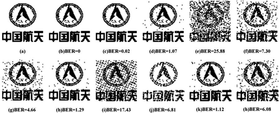
Fig. 5. Extracted watermark under various types of attack (a) None; (b–d) JPEG2000 compression with CR = 2, 4, 8; (e) Salt & pepper noise; (f) Median filter; (g) Gaussian filter; (h) Scaling; (i) Rotation; (j) Cropping; (k) Brighten; (h) Darken;
