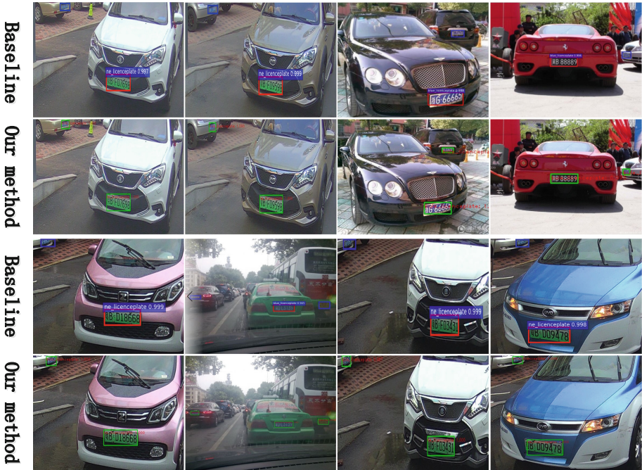
Fig. 4. Comparison of results. The first line is the baseline method test result picture, in which the blue rectangle represents the undetected object, the second line is our method test result picture.
