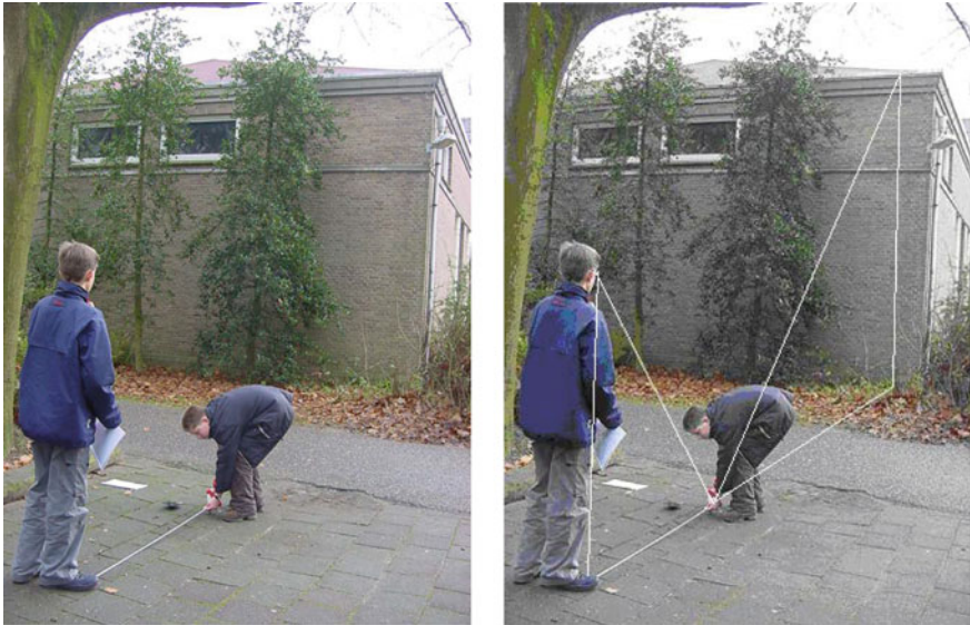
Fig. 13.6 Stefan sees the edge of the roof in mirror C; Marco measures Stefan’s distance from C
