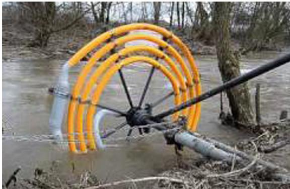
**Fig. 6.** Water wheel pumps
