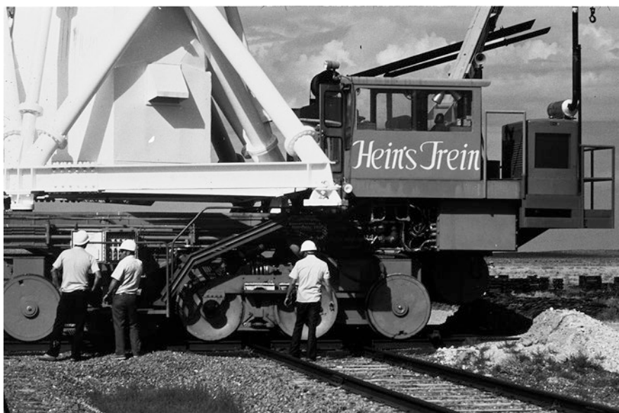
Fig. 7.8 Hein’s Trein, used to transport the VLA 25 meter antennas when reconfiguring the array. Credit: NRAO/AUI/NSF
