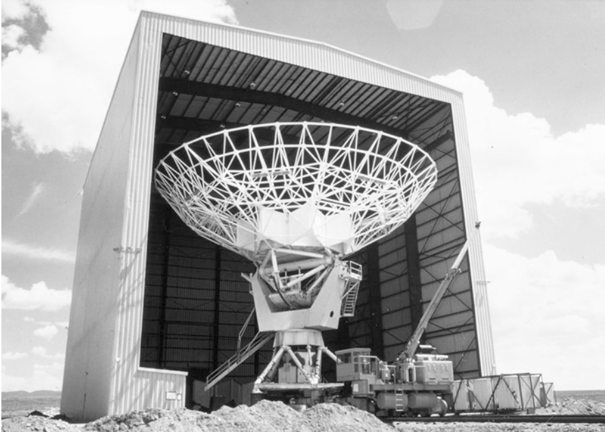
Fig. 7.11 First VLA antenna emerges from Antenna Assembly Building in July 1975. Credit: NRAO/AUI/NSF
