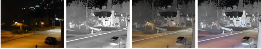
Fig. 6. Synchronized frames of video stream 15 from Camel [9] in the (from left to right) visual, infrared, addition and l1-norm subsets, favouring the fused subsets.
