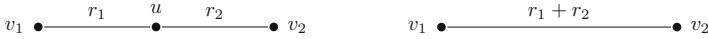
Fig. 2.4 An example of a network G where edges in series are replaced by a single edge
