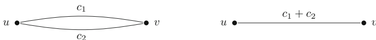
Fig. 2.3 Demonstrating the parallel law. Two parallel edges are replaced by a single edge
