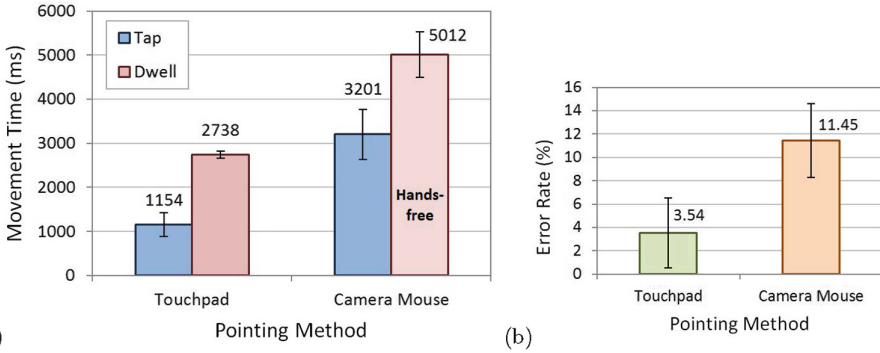
Fig. 7. Results for speed and accuracy (a) movement time by pointing method and selection method (b) error rate by pointing method with tap selection.
