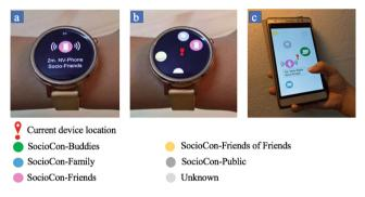
**Fig. 5.** Detailed view of a nearby device on the smartwatch screen (a), proximate selection map of nearby devices on the smartwatch (b) and the phone (c). This map shows each potential partnership device as a circle containing a device icon. The size of each circle is determined by the distance from the candidate to the current device. The circle color denotes its social relationship to the current device. (Color figure online)
