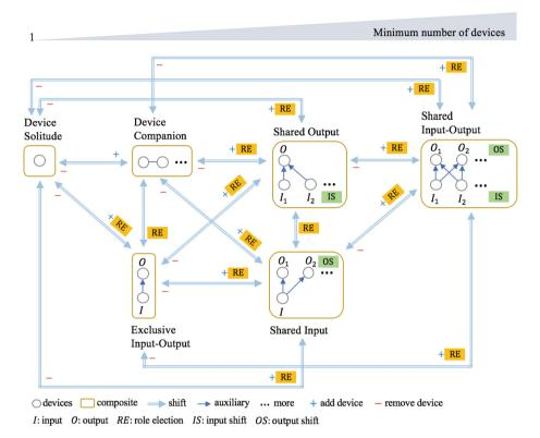
**Fig. 1.** Bi-directional shifts between device composites involve either the addition (+) or removal (-) of device(s), followed by Role Election (RE) in some cases. Input Shift (IS) and/or Output Shift (OS) take place within the device composites having shared input and/or output device(s).
